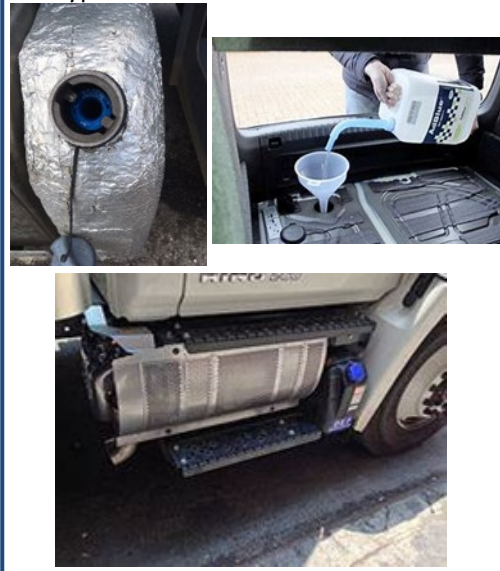
Typical truck mounted DEF reservoirs
